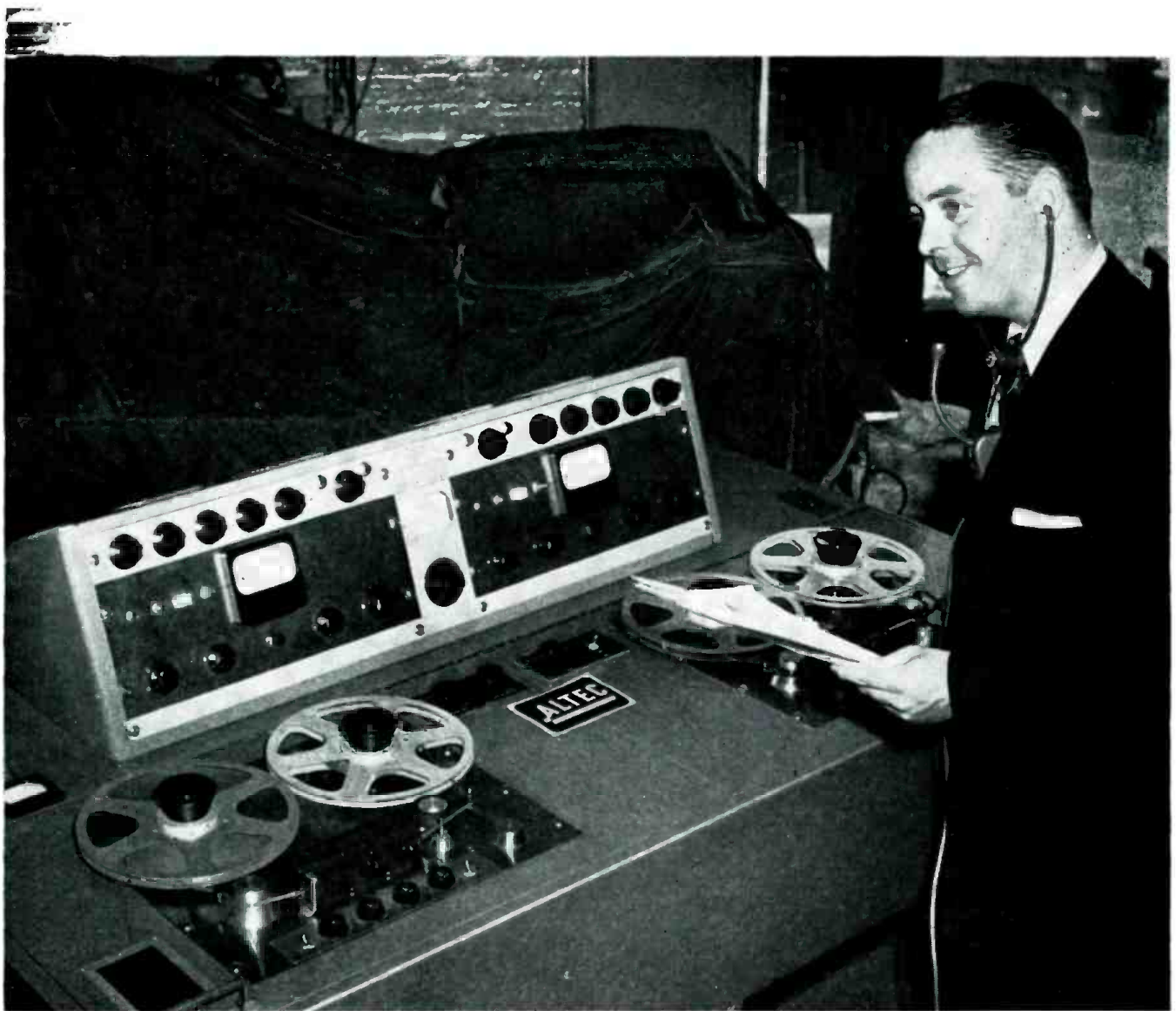
Equipped with a head set and chest plate mike, Wayne Thompson, master of ceremonies of "Holiday on Ice" operates the Cyclosonic audio control console. The unit has a dual amplification system permitting interchangeability in case of a component failure.
